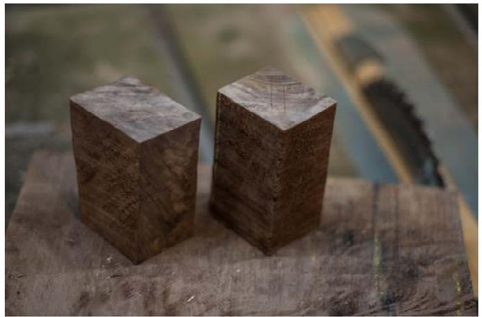
4-inch blocks ready to be drilled and mounted on mandrels
